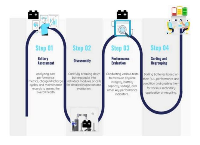
Figure 2: Battery Inspection Process.
